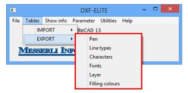
DXF (AutoCAD) and ELITECAD differ in the assignment of pen number and colour. In addition, ELITECAD has 1024 pens whereas DXF only has 256.
