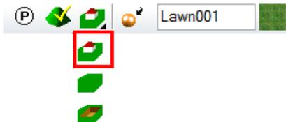
2. Start the TERRAIN function and then the function NEW TERRAIN EDGE/AREA. Ensure that the "type of entry" is set to contour entry.
