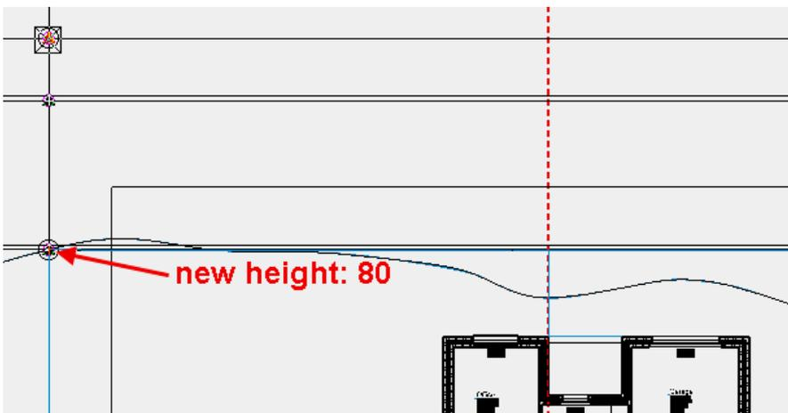
10. New heights must now be assigned to the terrain surfaces. Start the function NEW DEFINITION POINT.
