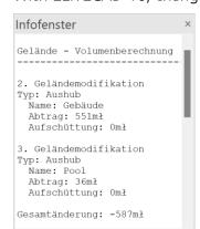
be listed in detail. The information window shows the amount of soil removed and applied for each modification. So that the individual work steps can be distinguished, the log also
