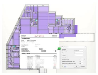
Depending on the project and storey options, ELITECAD Architecture 16 automatically calculates developed areas such as the building coverage ratio (BCR) and floor area ratio (FAR). You can easily select these in the quantity manager and check the associated total and individual areas and rules graphically.
