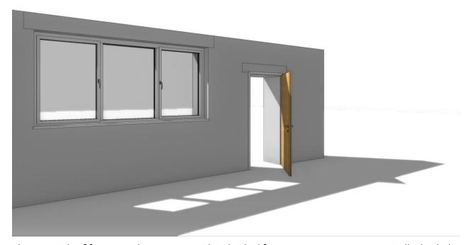
The materials of frames and casements with individual frame contours are automatically divided in the middle and the resulting contours are assigned the corresponding materials. Furthermore, corner stands in corner windows are considered as well. They are divided with the same plane as the frames. Mullions share the same material properties as the frames. For windows, the frame overrides the mullions, for glass elements they can be configured individually.
