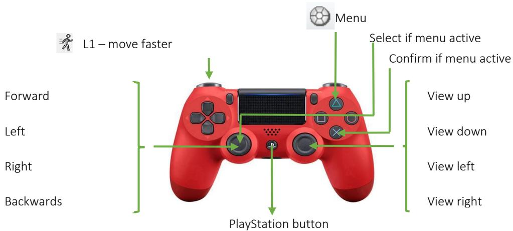
It is important to note that, in contrast to the keyboard, the amount of movement of the joystick controls the speed of the movements. This means, if the joystick is moved to the maximum, the speed will be much higher, than if it is moved just a little bit. Furthermore, it is possible to move both joysticks at the same time, which for instance allows moving forwards and at the same time changing the viewing direction.
